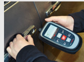
Testing a transmitter of a passive entry system
