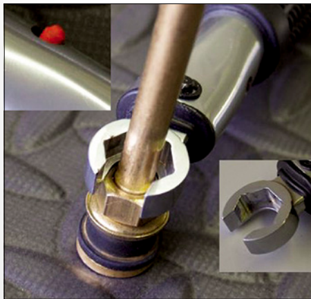
The Valve Nut Torque Wrench in use.
