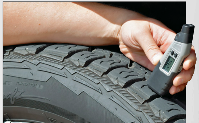
The Bartec TPG100 Tread Depth/Pressure Gauge in use.
