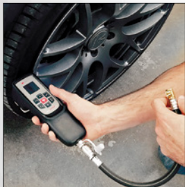
Testing the Bartec Tech200Pro TPMS Tool
